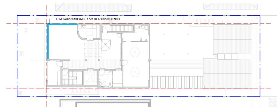
2 FIRST FLOOR PLAN FENCE / BARRIER DIAGRAM
