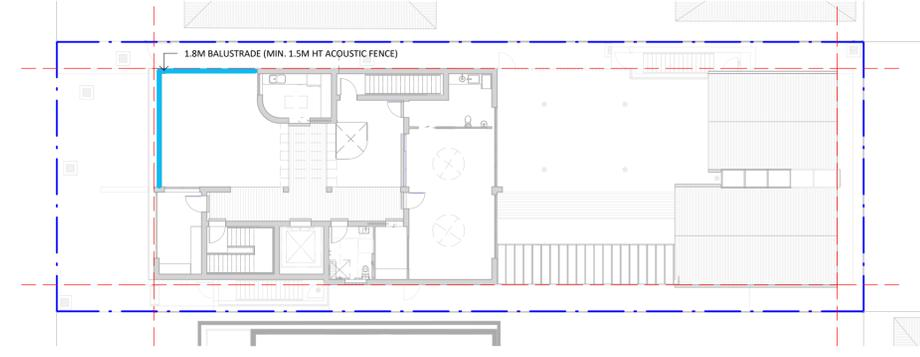
2 FIRST FLOOR PLAN FENCE / BARRIER DIAGRAM
